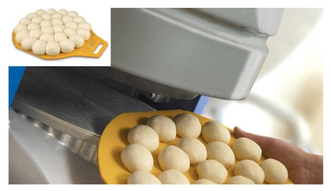
**DR** Fixed dividing disc, manual pressing and dividing, powered rounding
